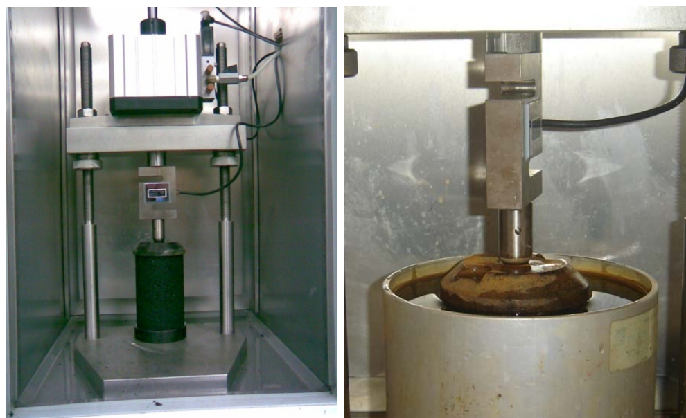
Figure 3-3 Flow Number Test Setup
